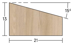
▲ Glazing bead For unrebated screen frames.
