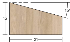
Glazing bead For unrebated screen frames.
