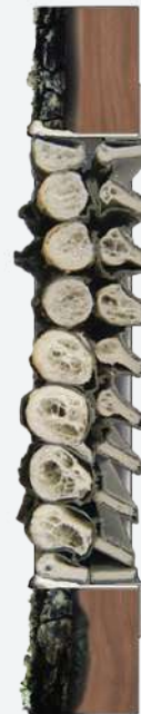
LVN20 air transfer grille in hot condition, showing intumescent material expanding to fill the space in the door
