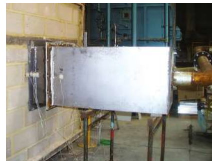
AS1530.4 2014 air transfer grille testing
